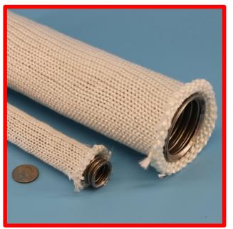
This Knitted fiberglass sleeve is fabricated from high quality type E fiberglass that will not burn and will withstand continuous exposure to temperatures of  $1200^{\circ}$ F /  $648^{\circ}$ C.
